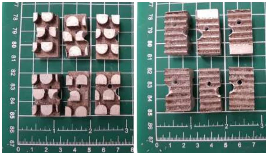
Figure 3: Pre-test images of the WB5 specimens tested in condensate A to F (left to right, top to bottom).
