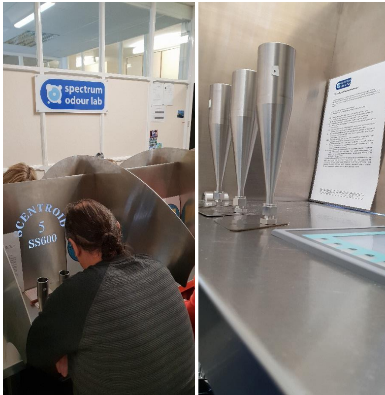
Figure 3: Olfactory testing with the five odorants in hydrogen mixtures performed at Air Spectrum
